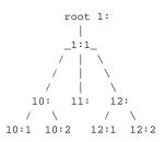
When enqueueing a packet, at each branch the filter chain is consulted for a relevant instruction. A typical setup might be to have a filter in 1:1 that directs a packet to 12: and a filter on 12: that sends the packet to 12:2.
